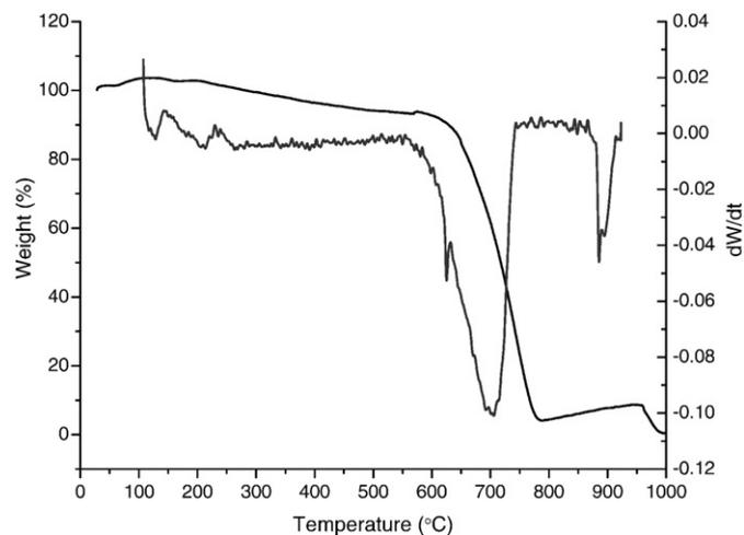
Fig. 3. TGA and DTGA curves of CNTs grown with natural palm oil.
