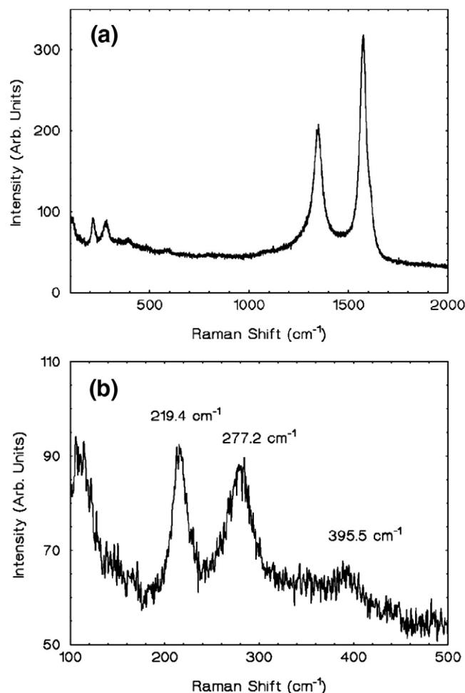
Fig. 2. Vibrational spectroscopy of VACNT grown with natural palm oil. (a) Microraman spectrum showing the RBM modes, the D line and the G line of CNTs. (b) Microraman spectrum showing the RBM modes of SWNT.
