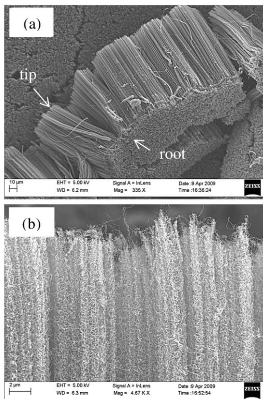
Fig. 1. FESEM images of VACNT grown on a Si substrate, (a) peeled off bundle of dense CNT, (b) side view of the aligned CNTs.
